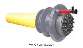
The "M" system is designed to comply with the guidelines ETAG 013 and it is awarded with the European Technical Approval ETA-09-0012 and the marking CE 0969-CPD-001/09-PT. The anchorage is made of: an anchor plate, wedges, connection and anchor casting. Simulations made with finite element codes and laboratory tests allowed to design a compact anchorage to comply with the guidelines ETAG 013.
