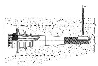
The removed and properly treated cap can be reused on several anchorages
