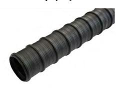
**SP** polyethylene sheaths are available in several versions. They are made of extruded H.D.P.E. according to the FIB Specification, in bars with a length from 5.8 m. to 11.8 m. They are blue with a heat-shrinking sleeve on each connection.
