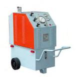
(Tensioning of TTM and M multi-strand anchorages)
