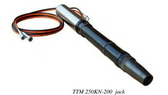
TTM 250KN-200 jack for tensioning on anchorages: E, EX and TTR provided with 200 mm actual stroke, hydraulic locking and tubes with 4 m quick joints.
