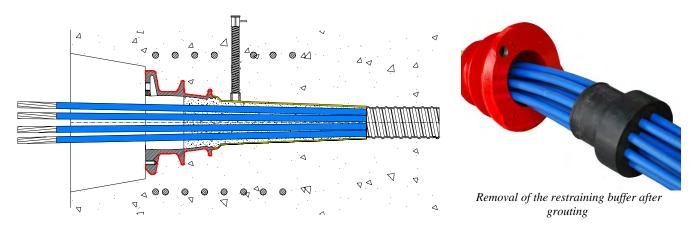
After grouting the buffer must be removed, thus obtaining a recess for the grease to protect the under plate strands.
