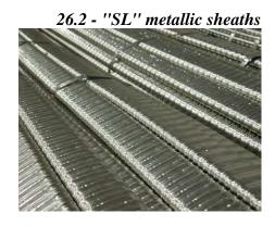
**SL** metallic sheaths are available in different versions. They are made of crimped sheet EN 10139 - 1999. They can be galvanized. Sheaths are available in bars having a length of 5.8 m. They are not all provided with a sleeve screwed onto each bar obtaining their connection by overlapping.
