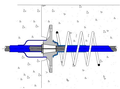
1E15 unbonded through anchorage with DD 1095GK gasket
