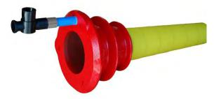
"M,  $M_{EP}$ " and MX"" anchorages are provided with a front grouting/vent hole which is placed on the highest point to guarantee a correct grouting by discharging any air. All castings are provided with protective covers for threaded holes to connect to the cap or to the formwork.
