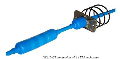
Unbonded 1GX15-C1 connection provided with a special protection outside the sleeve which allows it to slide while tensioning, thus guaranteeing a bonded/unbonded application. The sleeve protection must take into consideration the displacement of the sleeve during tensioning operations. The system protection relies on the two levels: grease and polyethylene, while the anchorage protection is obtained by means of passivation while grouting.
