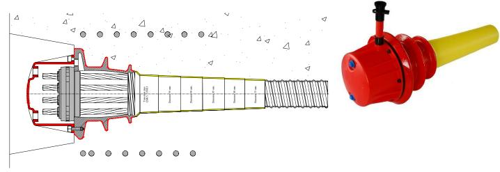
The "M" series active anchorage is made of the following parts: casting, anchor plate, wedges and connection in H.D.P.E. to connect the casting to the metallic or polyethylene sheath. Castings have a turned plane for the plate, holes for connection to cap and formwork and a threaded grouting hole. Castings are in spheroidal cast iron EN-GJS 500-7 EN-JS-1050, which offers a high resistance to stress. Being weldable, it guarantees the maximum safety during installation.
