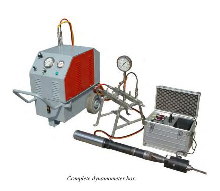
Capacity: 999 bar. Weight: 9.40 Kg./piece
