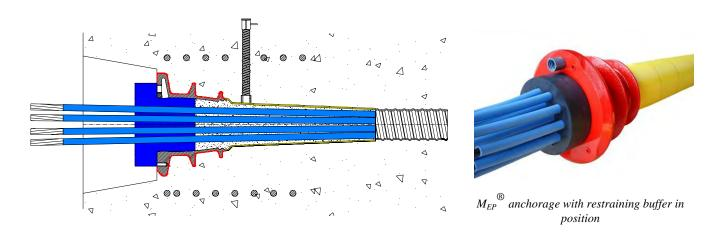
The buffer allows to restrain the grouting at half anchorage, allowing the insertion into the thus obtained recess of the greased anchorage to protect the uncovered strands.
