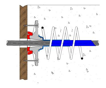
1EX15 unbonded anchorage with DD 1096GK gasket
