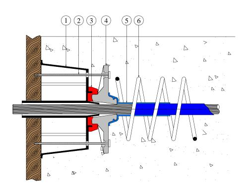
The 1E15 unbonded active anchorage with DD-1097A rectangular pocket former and DD 1095GK sealing gasket is made of the following parts: **Ref. 1** DD-1097A rectangular pocket former, **Ref. 2** fixing screws, **Ref. 3** DD 1095GK sealing gasket **Ref. 4** 1E15 steel anchor plate, **Ref. 5** rear connection and **Ref. 6** spring steel reinforcement,
