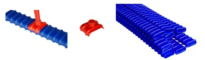
SPE-78x25x2 mm. polyethylene sheaths are made of extruded H.D.P.E. according to the FIB Specification, in bars with a length from 5.8 m. to 11.8 m. They are blue with a heat-shrinking sleeve on each connection.
