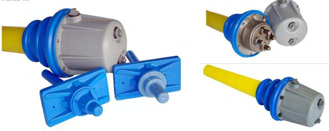
The application of X anchorages may be unbonded or bonded with grouting of cement or grease. The encapsulation of the whole anchorage with minimum 3mm polyethylene thickness allows a strong encapsulation of the device, which prevents corrosive agents from affecting its durability and effectiveness. The effectiveness of the system is completed by the use of polyethylene corrugated sheaths which guarantee the encapsulation of the whole cable.
