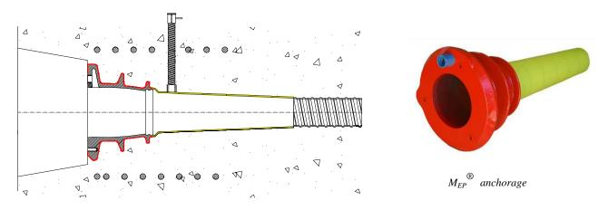
Grouting with vent placed on the truncated cone reduction in polyethylene of the  $M_{EP}^{(\mathbb{R})}$  anchorage
