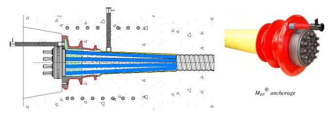
Insertion of the protection cap to guarantee the complete coverage of the anchorage area and its protection against corrosion.
