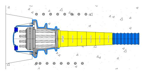
The resulting anchorage is used together with the casting versions  $M_{EP}$  and MX encapsulated and protected, in particular in the most complete version MX completely encapsulated in polyethylene.
