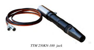
TTM 250KN-100 jack for tensioning on anchorages: E, EX and TTR provided with 100 mm actual stroke, hydraulic locking and tubes with 4 m quick joints.
