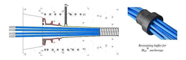
Insertion of greased and polyethylene-covered strands into the  $M_{EP}^{\, \otimes}$  anchorage. The restraining buffer allows to carry out the cable grouting before installing the anchor plate to block the strands.
