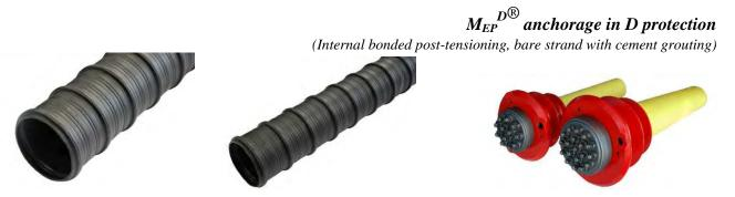
$M_{EP}^{D^{\circledR}}$  anchorage in D protection for <u>internal bonded post-tensioning</u>, made of: <u>casting protected with epoxy coating</u>, anchor plate with wedges, polyethylene connection, <u>protection cap</u>, wedges and <u>polyethylene corrugated sheath</u>. The permanent protection cap allows to protect the anchorage by restraining the grouting and by preventing infiltration into the protection cement over time. The anchorage is protected against corrosion with D level.
