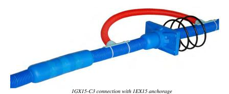
**Bonded 1GX15-C3** connection provided with a special protection outside the sleeve which allows it to slide while tensioning, thus guaranteeing a bonded/unbonded application. The sleeve protection must take into consideration the displacement of the sleeve during tensioning operations. The system protection relies on the two levels: grease and polyethylene for the cable, while the anchorage protection is obtained by means of a polyethylene encapsulation.
