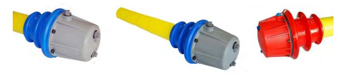
The DD-KP cap is made of polyethylene and together with a MEP or MX anchorage guarantees a double protection to corrosion. The DD-KP cap is provided with plugs to guarantee a correct grouting and vent when filling it.
