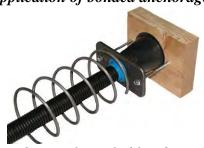
The rear connection guarantees a proper protection of the wire strand without polyvinyl chloride in the area of connection to the anchorage. The unbonded application can be carried out with a metallic sheath and a polyethylene sheath. Sheaths are provided with proper connections for grouting and vent to guarantee a correct grouting after tensioning.
