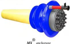
"MX <sup>®</sup>" series active anchorages are designed for post-tensioning applications in a <u>highly aggressive</u> environment. The anchorage is **completely encapsulated in polyethylene** on both casting and polyethylene cap to protect the anchor block, all grouted with grease.
