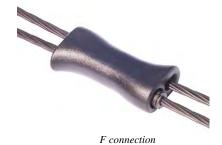
The F connection is used for the encircling of tanks or for the positioning into forming moulds as a tensionable connection of two strands. The anchorage is generally used as an unbonded active anchorage and it is used with greased and coated strands.
