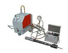
(Dynamometer for jack calibration)
