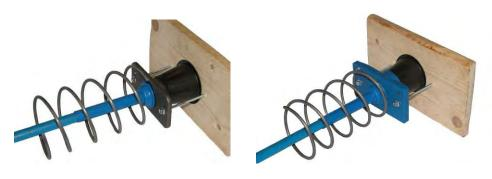
1E15 single strand anchorages are supplied with two holes to connect with the formwork. The anchorage of the steel plate to the formwork wood panel is guaranteed by two self-tapping screws.
