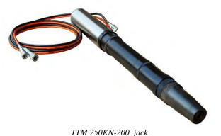
Weight: 26 Kg./piece Stressing section: 47.2 cm<sup>2</sup> Length: 950 mm. Max. diameter: 100 mm. Max. capacity: 250 KN Tensioning extension: 350 mm. Stroke: 200 mm. Provided with locking Type: **TTM 250KN-200**
