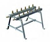
By means of a manifold, all the hydraulic pumps can be connected to several tensioning jacks. The **DD-MF** manifold is designed with 4, 6 or 10 hydraulic outputs under isopressure, it is made of galvanized steel and can be completely disassembled. The upper connections are for jacks, the side connections are for **TTM pumps**
