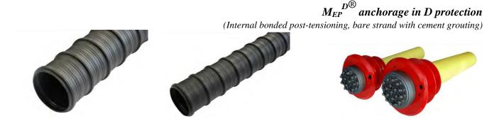
$M_{EP}^{D^{(k)}}$  anchorage in **D** protection for <u>internal bonded post-tensioning</u>, made of: <u>casting protected with</u> <u>epoxy coating</u>, anchor plate with wedges, polyethylene connection, <u>protection cap</u>, wedges and <u>polyethylene corrugated sheath</u>. The permanent protection cap allows to protect the anchorage by restraining the grouting and by preventing infiltration into the protection cement over time. The anchorage is protected against corrosion with D level.
