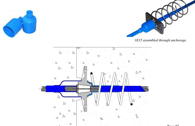
2.12 - 1E15-B unbonded anchorage with DD 7099B truncated cone pocket former
