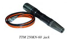
Stressing section: 47.2 cm<sup>2</sup> Length: 640 mm. Max. diameter: 100 mm. Max. capacity: 250 KN Tensioning extension: 350 mm. Stroke: 60 mm. Provided with locking Type: **TTM 250KN-60 jack**
