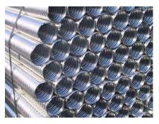
**ST** metallic sheaths are available in different versions. They are made of crimped sheet EN 10139 - 1999. They can be galvanized. Sheaths are available in bars having a length of 5.8 m. They are all provided with a sleeve screwed onto each bar.
