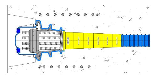
The resulting anchorage is used together with the casting versions  $M_{EP}^{\mathbb{R}}$  and  $MX^{\mathbb{R}}$  encapsulated and protected, in particular in the most complete version  $MX^{\mathbb{R}}$  completely encapsulated in polyethylene.
