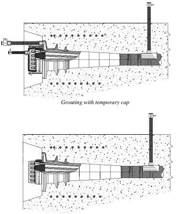
The removed and properly treated cap can be reused on several anchorages
