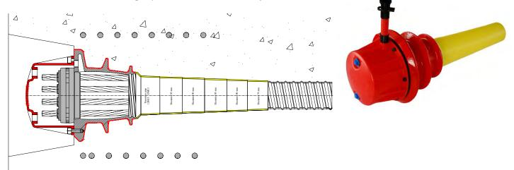
The "M" series active anchorage is made of the following parts: casting, anchor plate, wedges and connection in H.D.P.E. to connect the casting to the metallic or polyethylene sheath. Castings have a turned plane for the plate, holes for connection to cap and formwork and a threaded grouting hole. Castings are in spheroidal cast iron EN-GJS 500-7 EN-JS-1050, which offers a high resistance to stress. Being weldable, it guarantees the maximum safety during installation.
