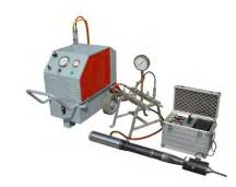
(Dynamometer for jack calibration)
