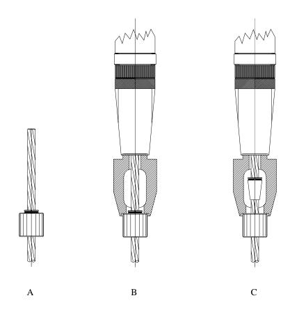
The releasing of wedges on M anchorages is carried out by means of TTM 2500KN-200-M jacks and of a TM 15 release cone.
