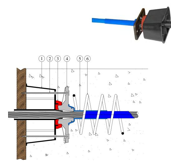
The 1E15 unbonded active anchorage with DD-1097A rectangular pocket former and DD 1095GK sealing gasket is made of the following parts: **Ref. 1** DD-1097A rectangular pocket former, **Ref. 2** fixing screws, **Ref. 3** DD 1095GK sealing gasket **Ref. 4** 1E15 steel anchor plate, **Ref. 5** rear connection and **Ref. 6** spring steel reinforcement,
