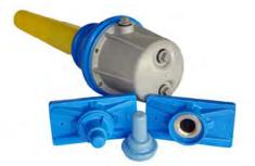
X series anchorages, both single and multi-strand, are encapsulated with polyethylene in order to guarantee unlimited durability and resistance against corrosion, provided the devices are properly installed. A layer of polyethylene covers the whole anchorage, allowing a grouting of cement or grease inside it.
