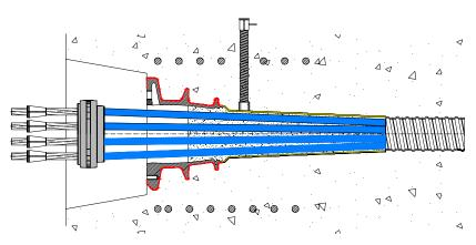
Approaching of the anchor plate and insertion of locking wedges.
