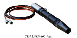
**TTM 250KN-100** jack for tensioning on anchorages: E, EX and TTR provided with 100 mm actual stroke, hydraulic locking and tubes with 4 m quick joints.
