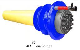
"*MX*<sup>®</sup>" series active anchorages are designed for post-tensioning applications in a <u>highly aggressive environment</u>. The anchorage is **completely encapsulated in polyethylene** on both casting and polyethylene cap to protect the anchor block, all grouted with grease.
