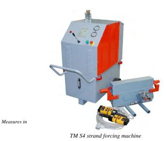
Pump weight: 380 Kg./piece Strand forcing machine weight: 80 Kg./piece
