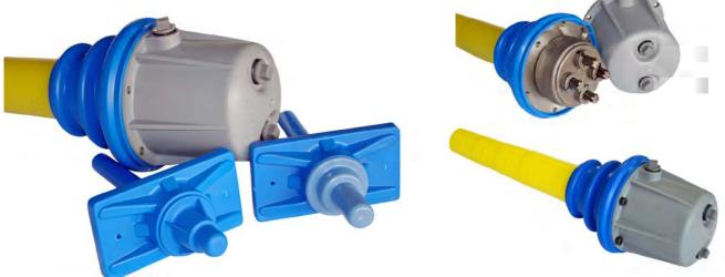
The application of X anchorages may be unbonded or bonded with grouting of cement or grease. Encapsulating the whole anchorage with a minimum thickness of 3 mm. of polyethylene allows a strong encapsulation of the device not to allow corrosive agents to compromise the durability of the device and its effectiveness. The effectiveness of the system is completed by the use of polyethylene corrugated sheaths which guarantee the encapsulation of the whole cable.
