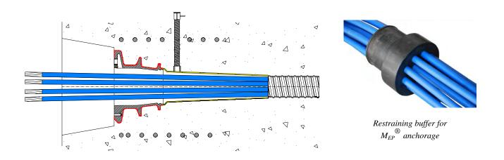
Insertion of greased and polyethylene-covered strands into the  $M_{EP}^{\otimes}$  anchorage. The restraining buffer allows to carry out the cable grouting before installing the anchor plate to block the strands.
