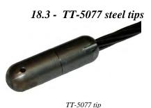
**TT-5077** tips are designed for very difficult threading. They are made of steel and provided with blocking with T15 wedges. In those cases where threading is very difficult and where the plastic tips break because of the roughness of the positioning of the sheaths, **TT-5077** steel tips are recommended because they offer a greater resistance to impacts.
