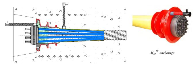
Insertion of the protection cap to guarantee the complete coverage of the anchorage area and its protection against corrosion.
