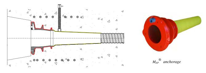
Unbonded post-tensioning application phases with the  $M, M_{EP}^{\mathbb{R}}$  and  $MX^{\mathbb{R}}$  devices.
