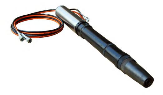
TTM jacks are available in three models which differ according to use characteristics. They are provided with an automatic locking circuit and 4 meter long flexible tubes. The main use of **TTM250KN** jacks is for tensioning on single strand heads on TTM anchorages. They are available with strokes: 400 mm., 200 mm., 100 mm. and 60 mm., the stroke reduction allows smaller dimensions of the jack.
