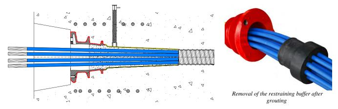
After grouting the buffer must be removed, thus obtaining a recess for the grease to protect under plate strands.
