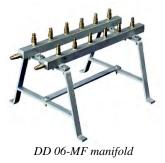
Useful positions: 6 outputs + gauge fix. Weight: 25 Kg./piece Dimensions: 800x500x410 mm Max. operating pressure: 450-500 bar.
