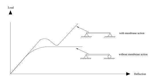
Effect of the bending stress on the slab load-bearing capacity
