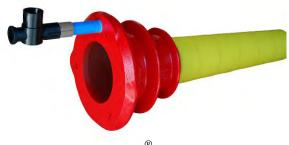
" $M, M_{EP}$ " and MX" anchorages are provided with a front grouting/vent hole which is placed on the highest point to guarantee a correct grouting by discharging any air. All castings are provided with protective covers for threaded holes to connect to the cap or to the formwork.
