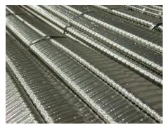
**SL** metallic sheaths are available in different versions. They are made of crimped sheet EN 10139 - 1999. They can be galvanized. Sheaths are available in bars having a length of 5.8 m. They are not all provided with a sleeve screwed onto each bar obtaining their connection by overlapping.
