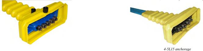
The 4-5L15 anchorage allows to install 4 and 5 strand anchorages that are encapsulated in polyethylene by installing a single anchorage that can be connected to the polyethylene-covered strands. It can be easily connected to the formwork and it is easy to install, grout and tension with a jack, strand by strand.
