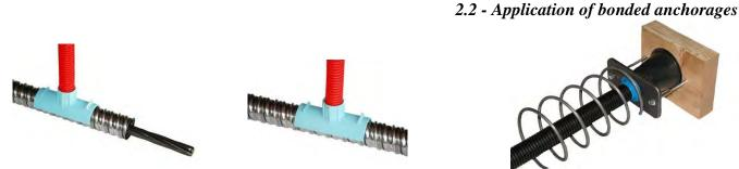
The rear connection guarantees a proper protection of the wire strand without polyvinyl chloride in the area of connection to the anchorage. The unbonded application can be carried out with a metallic sheath and a polyethylene sheath. Sheaths are provided with proper connections for grouting and vent to guarantee a correct grouting after tensioning.
