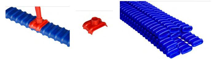
**SPE-78x25x2 mm.** polyethylene sheaths are made of extruded H.D.P.E. according to the FIB Specification, in bars with a length from 5.8 m to 11.8 m. They are blue with a heat-shrinking sleeve on each connection.
